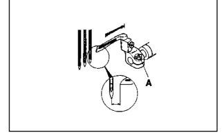
\* For easy adjustment of Looper movement to the right, use Timing Gauge (95220). As the Timing Gauge is optional, request it to the agent who sold the machine to you or directly to us.
