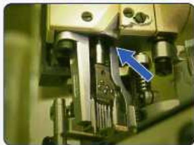
While giving enough lubrication for internal driving mechanism, Yamato exclusive sealing system prevents the oil from coming to sewing area through moving parts. This feature minimizes the risk of oil stain, one of the most frequent causes of defects.
