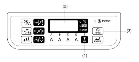
• The 4-column data in the display (2) can be changed to one of the following three statuses each time the SEL key (1) is pressed.
