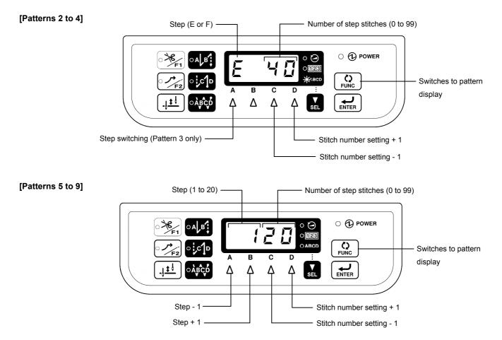
• The thread trimming disable/F1 key can be used to set the automatic thread trimming function. (Setting is possible for patterns 2 to 9.)
