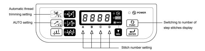
• The thread trimming disable/F1 key can be used to set the automatic thread trimming function. (This can be set for patterns 2 to 9.)
