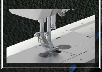
Upper thread holding device is equipped as standard
