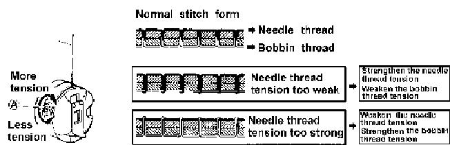
Thread tension should be determined in accordance with the stitches obtained by adjusting the tension of the bobbin thread and needle tension (Fig. 12).
