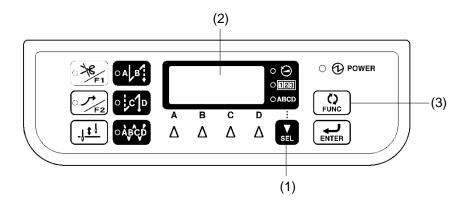
· 4 digits display can be changed by pressing SEL key (1) each time for three kind of condition.
