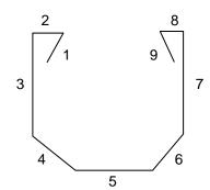
STEP1: Start backtacking A=4,B=4、Step stitches=5, AUTO mode
