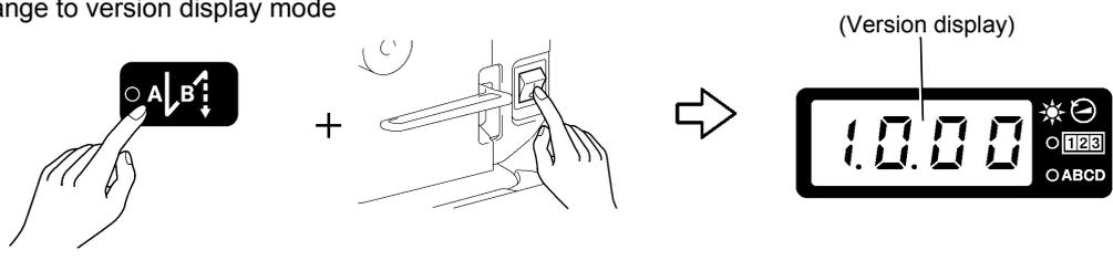
(While pressing the start backtack key, press the power ON switch.)
